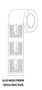
Standard Alien Inlay rolls unwind with metal antenna side facing outward, with respect to the core.
